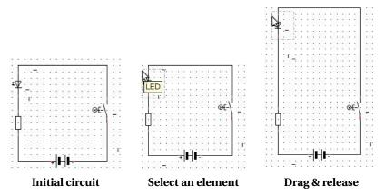
Adjusting connectors by moving element in a circuit
